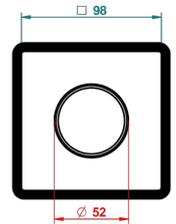
Tube / Pipe Joint Plaque / Seal Plate
