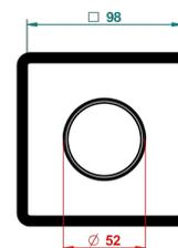
Tube / Pipe Joint Plaque / Seal Plate
