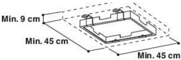
*Let a minimum reserve of 45X45X9 – Fix the ceiling support securely. Caution : respect imperatively the dimension of 5.3cm*
